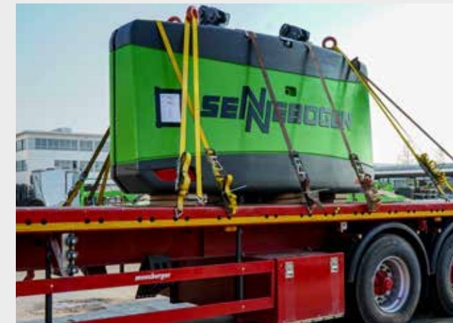
870 Demolition: Removable counterweight reduces transport weight
