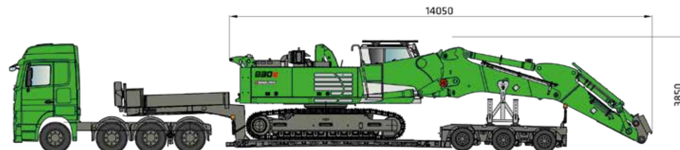
TRANSPORT OPTION BASE MACHINE + EA12, INCL. BEARING BASE, WITHOUT CONTAINER WEIGHT, APPLICATION WEIGHT: 51 t
