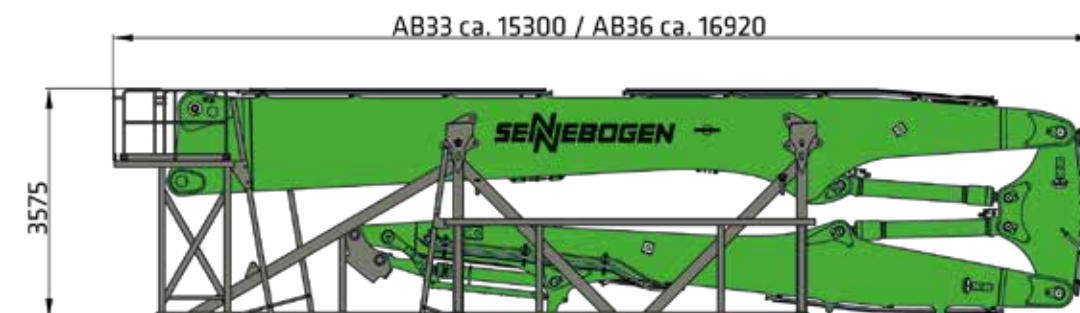
3-PART DEMOLITION BOOM INCL. TRANSPORT FRAME APPROX. 25 t – 28 t
