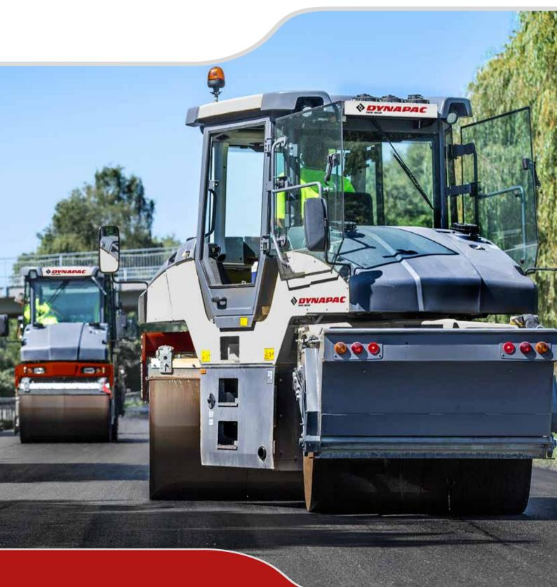
Instead of central articulation, machines in the Dynapac CG roller range traditionally have steering on the drums. Dynapac Road Construction Equipment is presenting the Dynapac CG2300, as a supplement to its articulated CC machines. The Dynapac CG2300 is 3.99 m long, 2.99 m high, has an inner turning radius of only 2.65 m and an off-set as big as 1.2 m, making it easy to transport and manoeuver in confined spaces.
