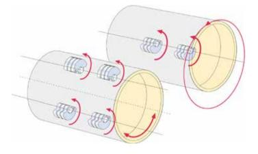
The Dynapac CO2200, CO4000 VI, CO4200 VI, CO5200 VI and CO6200 VI rollers have one vibrating drum with two vibration amplitudes and one oscillating drum. This allow the operator to select the system that is most suitable for the application on hand.
